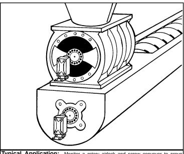
Typical Application: Monitor a rotary airlock and screw conveyor to prove rotation for interlocked material handling equipment.
